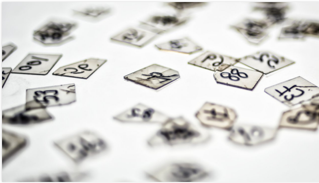
Lab diamonds start their life as small numbered plates, diamond discs also called 'seeds'. ©Debby Termonia
